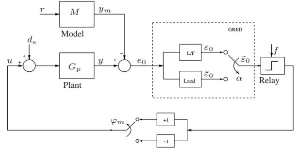
Fig. 1. VS-MRAC using a hybrid lead filter (GRED) for relative degree compensation and a switching scheme to adjust the control sign.  $LF$  and  $L_{red}$  stand, respectively, for the linear and nonlinear (RED based) lead filters.
