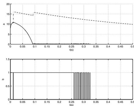
Fig. 3. Simulation results (Example 1); (a) monitoring function  $\varphi_m$  (dash) and the auxiliary error  $\tilde{e}_0$  (line); (b) switching function  $\alpha$ :  $\alpha = 1$  (linear lead filter) and  $\alpha = 0$  (nonlinear lead filter).
