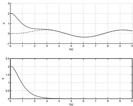
Fig. 2. Simulation results (Example 1). Simulated (a) plant output  $y$  (line), reference model output  $y_m$  (dash) and (b) the plant tracking error  $e_0$ .
