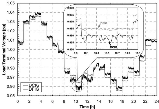
Figure 7 – Load voltage profile
