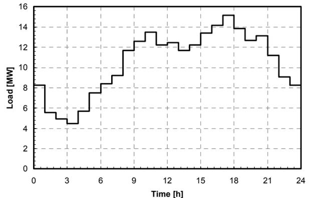
Figure 5 – Daily system load curve
