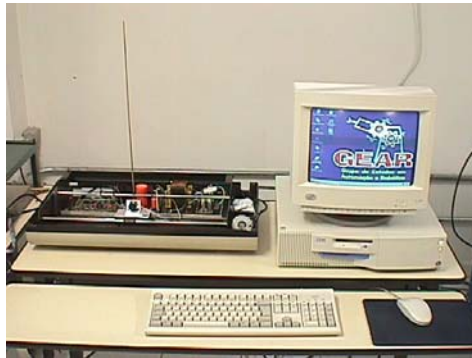
Figure 4. Inverted Pendulum testbed at PUC Minas.
