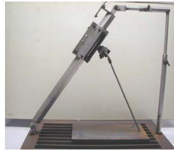
Figure 6 - Gravitational mechanized system for welding with covered electrodes
