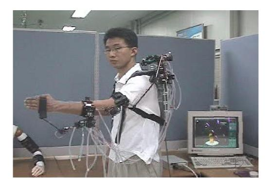
Prototype of the wearable teleoperation master is shown above. Small brakes for force reflection are achieved utilizing hydraulic cylinder with close loop control valve.
