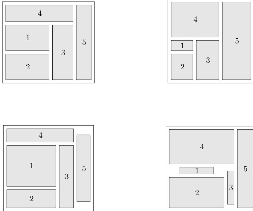
Figure 8.20 Four instances of an optimal floor plan, using the relative positioning constraints shown in figure 8.18. In each case the objective is to minimize the perimeter, and the same minimum spacing constraint between cells is imposed. We also require the aspect ratios to lie between 1/5 and 5 . The four cases differ in the minimum areas required for each cell. The sum of the minimum areas is the same for each case.
