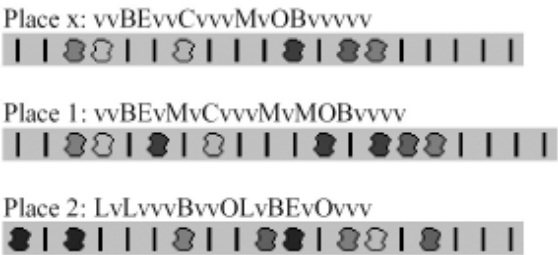
Figure 4.52 Three actual string sequences. The top two are strings extracted by the robot at the same position [95].
