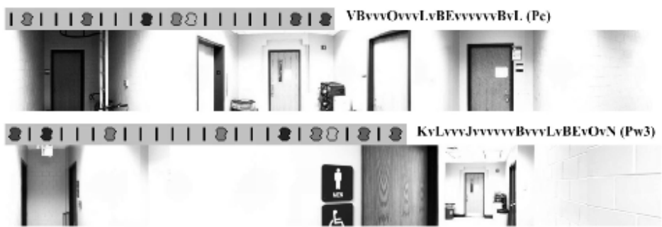
Figure 4.51 Two panoramic images and their associated fingerprint sequences [95].
