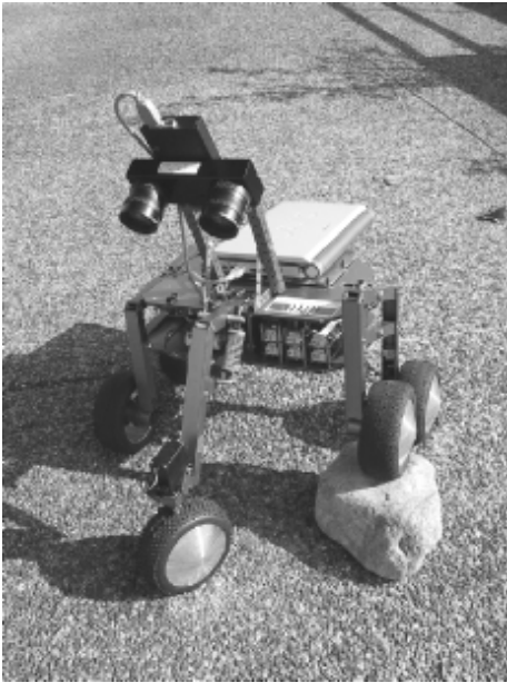
Figure 4.25 The SVM module mounted on EPFL's Shrimp robot.
