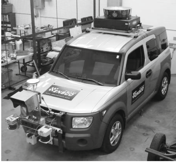
Fig. 1.6 A car-like robot developed by Team ENSCO for 2007 DARPA Urban Challenge Source: http://en.wikipedia.org/wiki/Image:ElementBlack2.jpg
