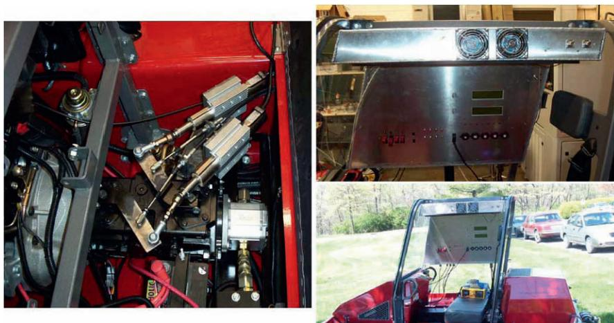
**Fig. 1.6** MARVIN II's actuator setup for autonomous navigation (left), and custom control box housing the embedded controller and other components (right).
