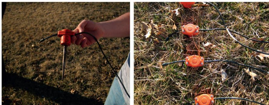
**Fig. 1.14** Spiked geophone (left), and several deployed by inserting the spikes into the surface (right).
