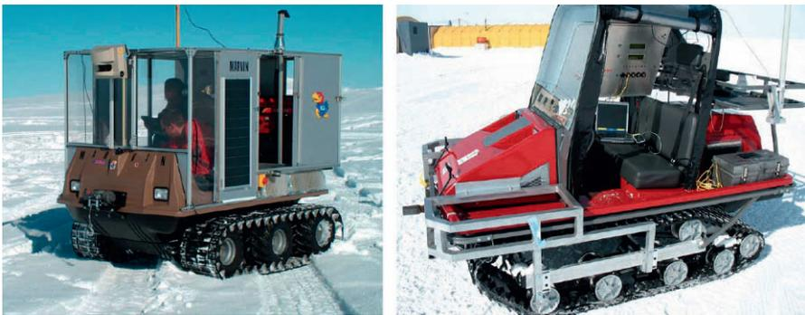
**Fig. 1.1** MARVIN I (left, in Greenland) and MARVIN II (right, in Antarctica) equipped with components for polar operations.
