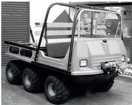
**Fig. 1.3** Original Buffalo Max ATV used as the base platform for the MARVIN I mobile robot.
