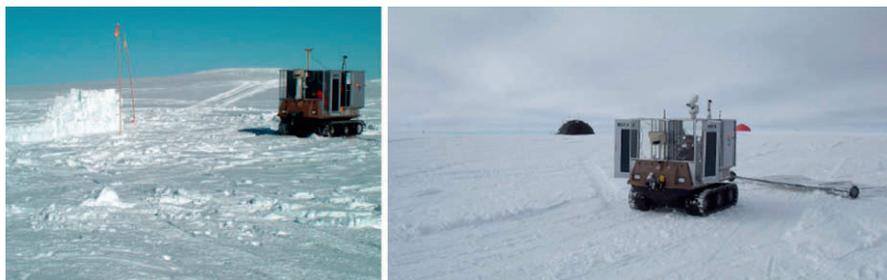
Fig. 1.11 Evaluation of MARVIN I systems at North GRIP, including using a laser range-finder to image a snow wall (left) and towing a mockup radar array (right).
