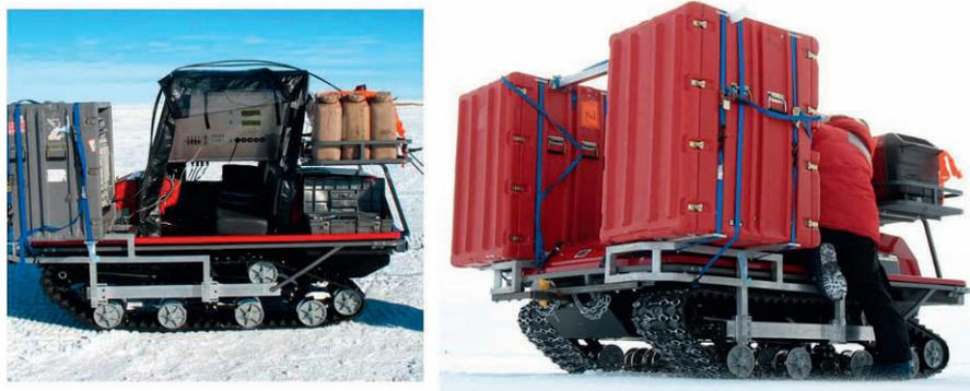
**Fig. 1.7** MARVIN II platform with environmental enclosure, radar crate mounted on the front, and additional fuel on the back (left); and larger crates mounted on both sides of the custom aluminum frame (right).
