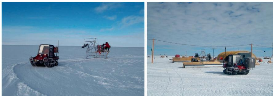
Fig. 1.12 MARVIN II rover towing a radar sled for a mono-static application (left) and a radar sled for a bi-static application (right) in Antarctica.
