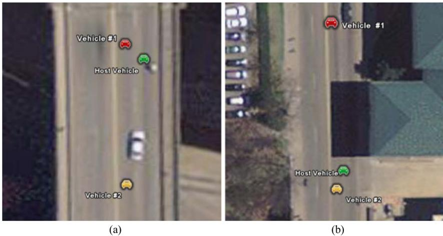
**Fig. 8.8** Mapping from detected objects onto Google Earth map: (a) The objects are detected from the top image in Fig. 8.1; (b) The objects are detected from the bottom image in Fig. 8.1
