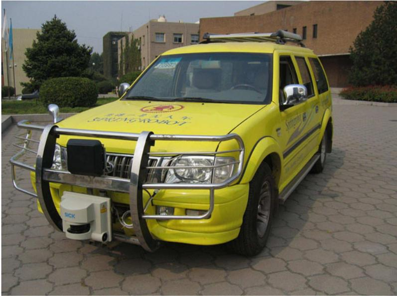
Fig. 6.5 Intelligent driver assistance and safety warning platform—Springrobot
