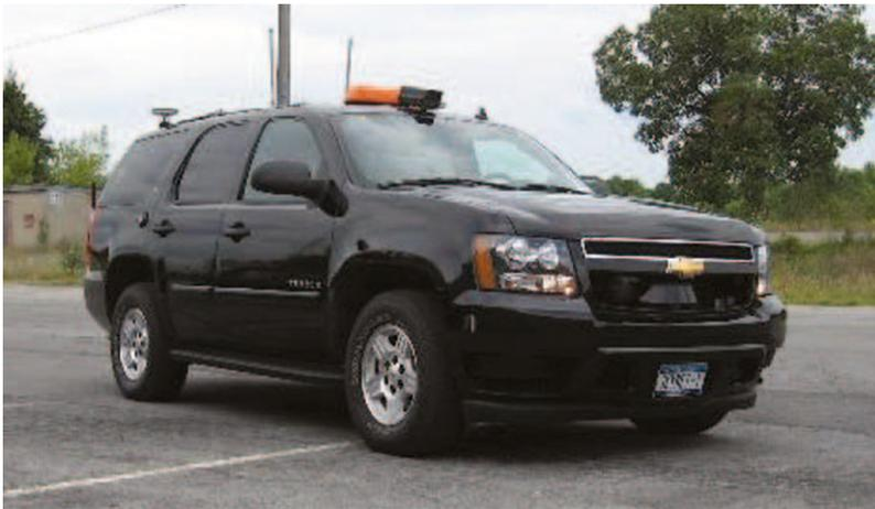
**Fig. 2.5** The intelligent vehicle Skynet developed by Team Cornell (published courtesy of Cornell University)
