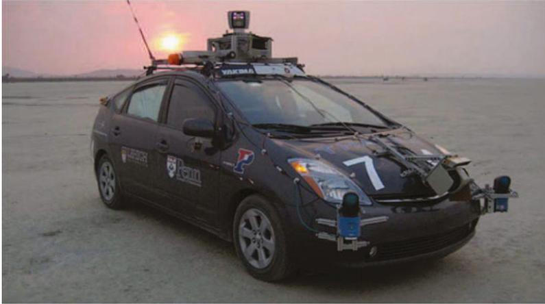
**Fig. 2.6** The intelligent vehicle Little Ben (published courtesy of the University of Pennsylvania and Lehigh University)
