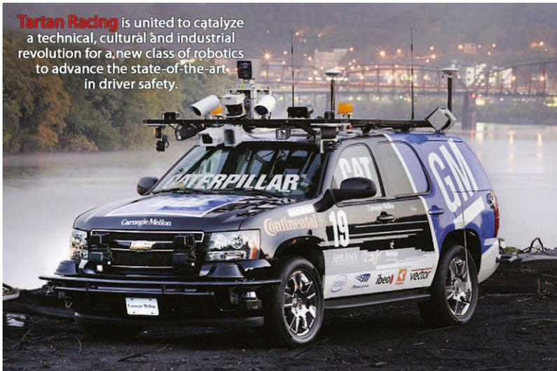
**Fig. 2.1** The intelligent vehicle, named Boss, developed by Carnegie Mellon University's Red Team (published courtesy of Carnegie Mellon University)
