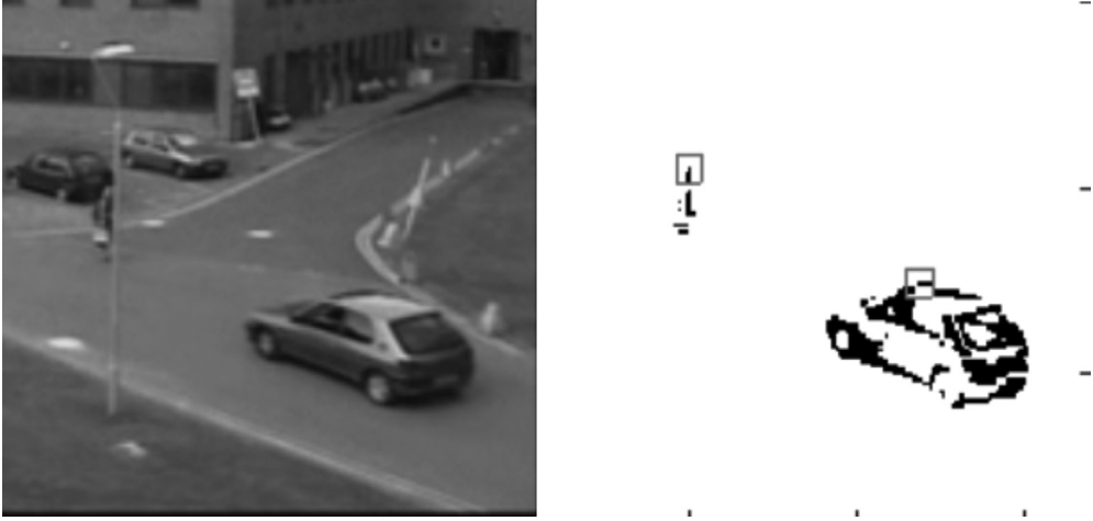
Figure 13.6 Background subtraction using RDE method, Left-hand side plot represents the scene in which there are two moving objects new to the scene; right-hand side plot represents the foreground in black and the background in white. The squares denote the focal points of the physical objects identified to be moving (the car and the pedestrian, respectively)
