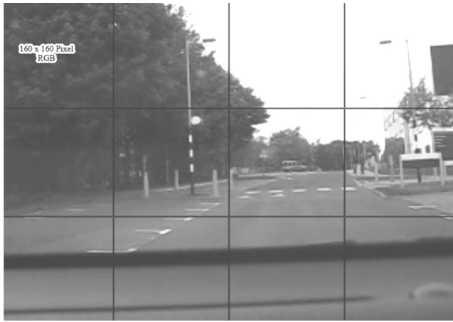
Figure 12.6 Image (with size 640 \times 480 pixels) segmented into 12 bins with size 160 \times 160 pixels
