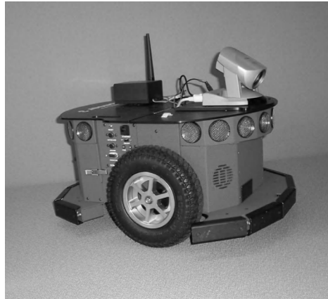
Figure 12.1 Mobile robot Pioneer 3DX used in the experiments at Infolab21, Lancaster University, UK
