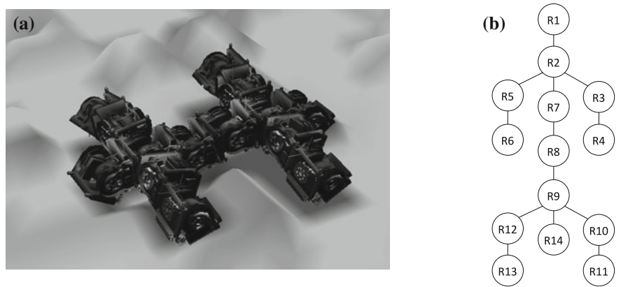
Fig. 4.7 REPLICATOR modular robotic organism. a Modular robotic organism comprising 14 robotic modules, b Morphology graph
