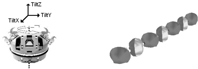
Fig. 5 From left to right: An ATRON module, a seven-segment snake robot
