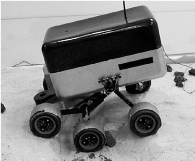
Fig. 4.9. Experimental rover during go/no-go ditch traversal experiment
