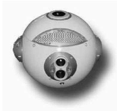
Figure 1.1 NASA's Mini AERCam free-flying video inspection robot.
