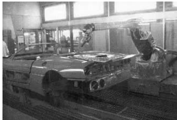
Figure 1.5 ABB painting robot named Tobe.
