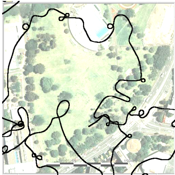
Figure 12.13 The testing environment: A 350 meters by 350 meters patch in Victoria Park in Sydney. Overlaid is the integrated path from odometry readings.
