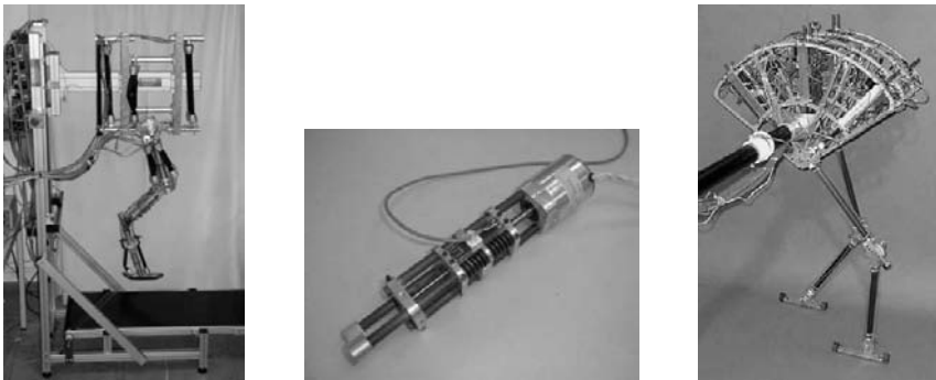
Fig. 2. (a) PANTER leg – (b) Series Elastic Actuator – (c) Spring Flamingo
