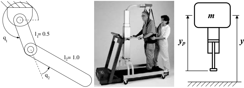
Fig. 1. The left-hand system was used for Case 1, a fully actuated robot. Case 2 is the same system, but with the base joint unactuated. The center system represents Case 3, which is an application to human step rehabilitation. The right system is a hopping machine for Case 4
