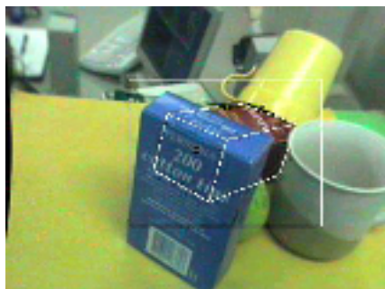
(a) Frame 670: pose biased by distracting edges in occluding objects
