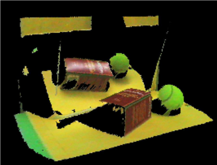
Fig. 3.12. Robust scanner results in the presence of secondary reflections (see Multimedia Extensions for VRML model). Reprinted from [151]. ©2004, Sage Publications. Used with permission.
