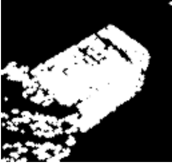
(b) Output of colour filter applied to current frame ROI
