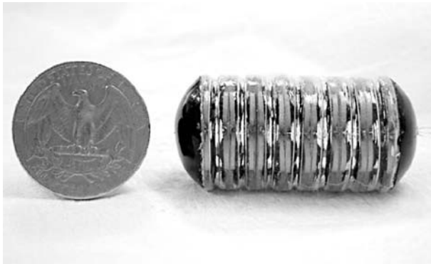
Figure 3.35. An inchworm robot
