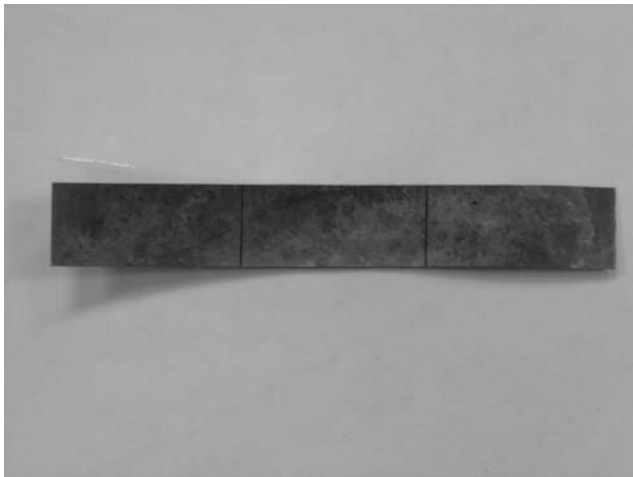
Figure 10.2. IPMC with three segment design
