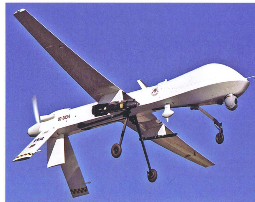
Unmanned and unafraid. The first hunter-killer UAV was the MQ-1B Predator, a modified version of the RQ-1 Predator reconnaissance drone, adapted to carry the AGM-114 Hellfire laser-guided missile. It has been used in combat in Iraq, Afghanistan, Yemen, and other locations. (USAF)
