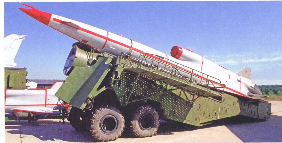
The VR-2 Strizh was based on the Tupolev Tu-141 drone and was launched using rocket assist from this SPU-141 semitrailer launcher. (Author)
