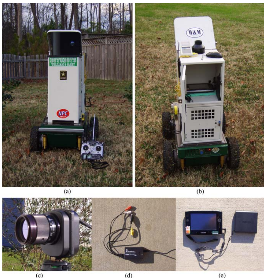
Fig. 2.1 Robotic thermal imaging system hardware: (a) robot platform front view, (b) robot platform rear view, (c) Raytheon thermal imaging video camera, (d) VideoAdvantage USB video capture device, (e) Samsung tablet PC w/ Powerbank.
