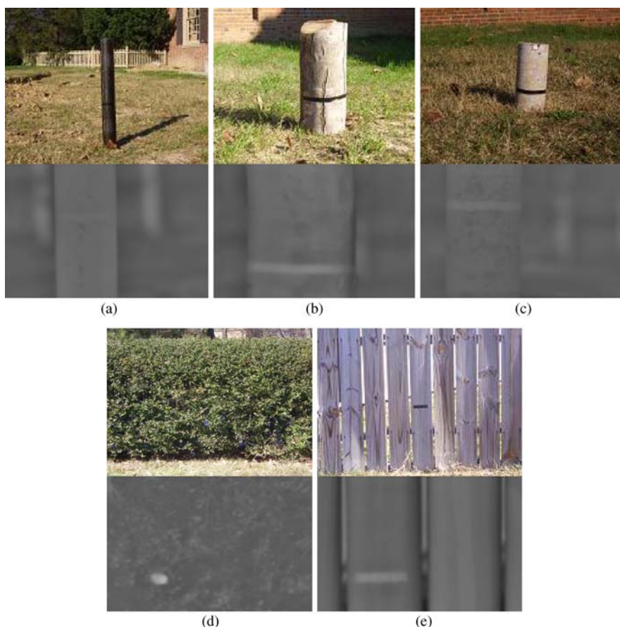
Fig. 3.9 Visible and thermal images of objects captured on 10 February 2007 to evaluate the emissivity feature. (a) steel pole, (b) birch tree log, (c) concrete cylinder, (d) hedges, and (e) wood wall.
