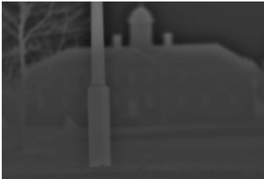
Fig. 2.10 Thermal image with preprocessing on temporal/spatial signal degradations and dead pixels. AGC is disabled.
