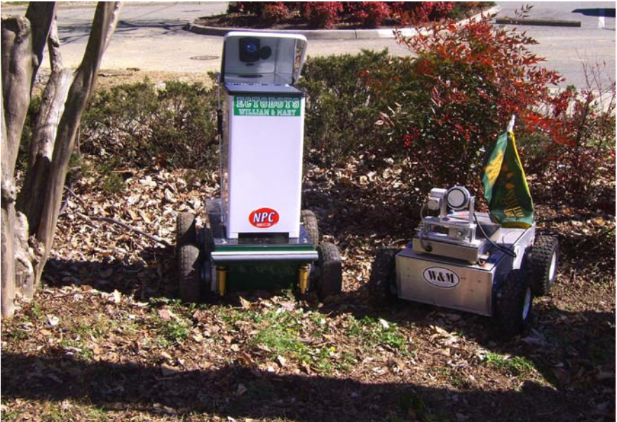
Fig. 1.3 Mobile robotic 3D sonar scanning system, rWilliam (on right) and thermal imaging system, rMary (on left).
