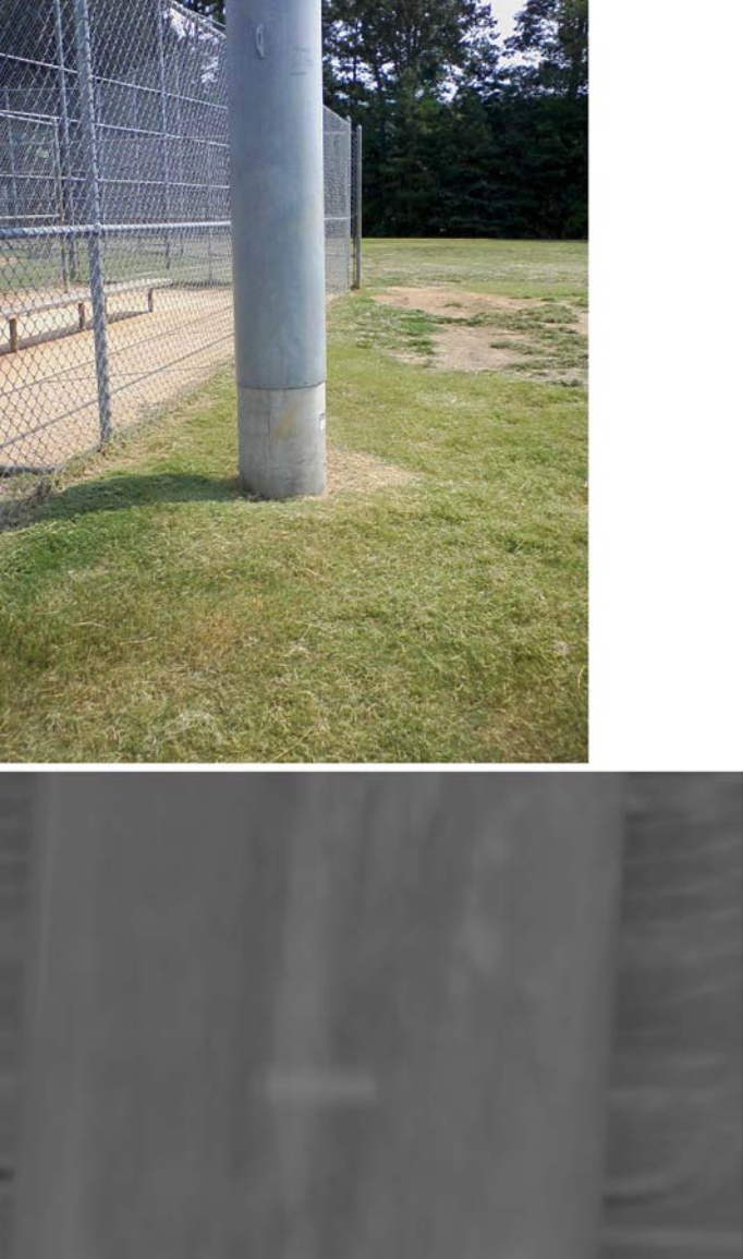
Fig. 5.12 Visible and thermal images of a steel pole from the blind data set that was misclassified as a tree by the adaptive Bayesian Classifier. The thermal image was captured on 5 November 2007 at 1428 hrs.
