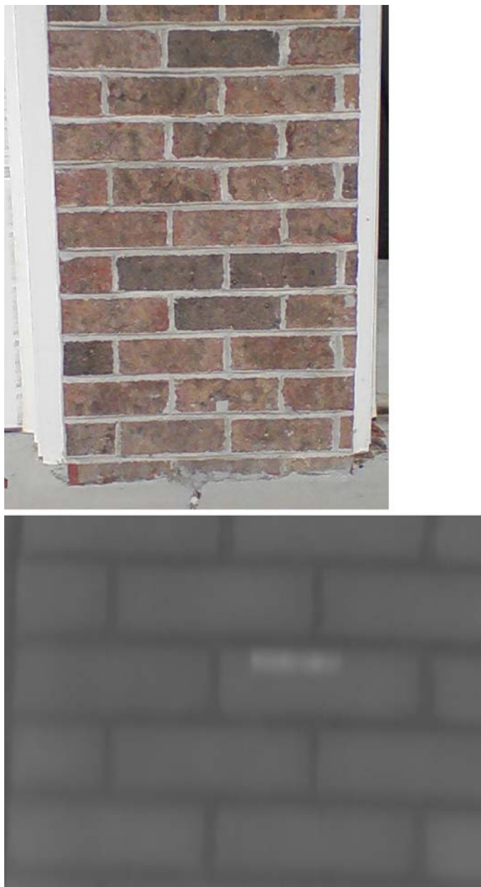
Fig. 5.7 Visible and thermal image of brick wall from the blind data set that was misclassified as a hedge by the adaptive Bayesian classifier. The thermal image was captured on 24 September 2007 at 1005 hrs.
