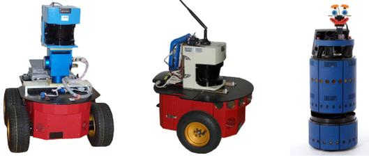
**Fig. 6.4.** Different types of robot used to acquire real robot data used for mapping (ActivMedia Pioneer 2 AT, Pioneer 2 DX-8, and an iRobot B21r).
