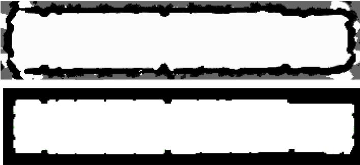
**Fig. 3.4.** The top image depicts a coverage map learned from ultrasound data using our sensor model and map update technique. In this experiment, most of the obstacles fit into the grid discretization and therefore only a few cells show partly occupied cells. The lower image illustrates the corresponding ground truth map learned from laser range data.
