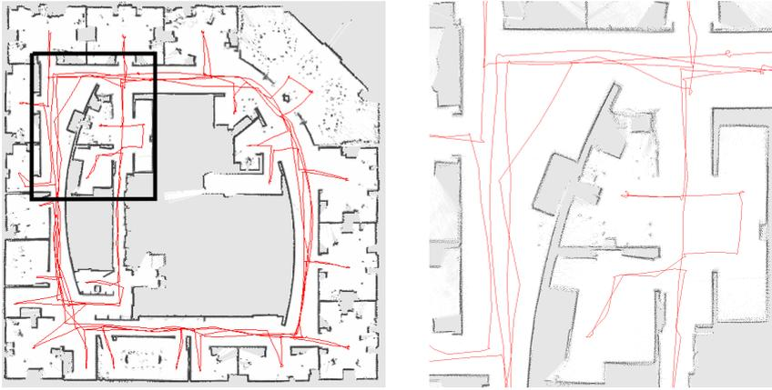
**Fig. 6.5.** The Intel Research Lab: The robot starts in the upper part of the circular corridor, and runs several times around the loop, before entering the rooms. The left image depicts the resulting map generated with 15 particles. The right image shows a magnified view with a grid resolution of 1 cm to illustrate the accuracy of the map in the loop closure point.
