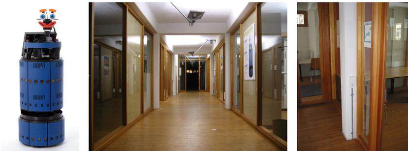
**Fig. 3.5.** The left image depicts the B21r robot Albert used to carry out the experiments. Albert is equipped with ring of 24 ultrasound sensors. The other images show photographs taken within the corridor of our office environment.
