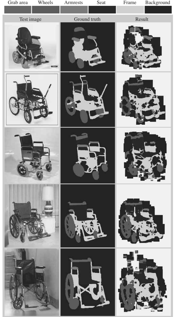
Fig. 4. Results for the annotation verification experiment on wheelchair images. From left to right: test image, ground-truth, and output of our system. White areas are unlabeled and can be considered background.
