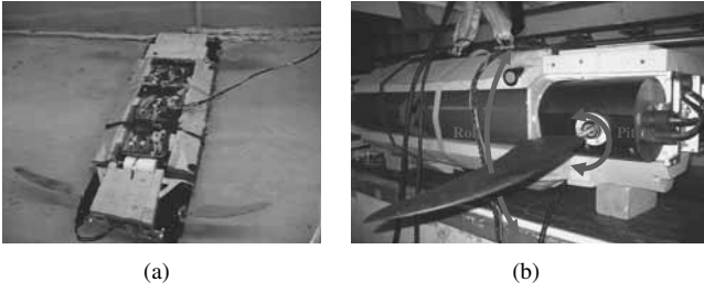
Fig. 1. “The biomimetic flapping foil autonomous underwater vehicle (BFFAUUV) was conceived as a test platform and proof of concept for the use of flapping foils as the sole source of propulsion and maneuvering forces in an underwater vehicle,” quoting [12]
