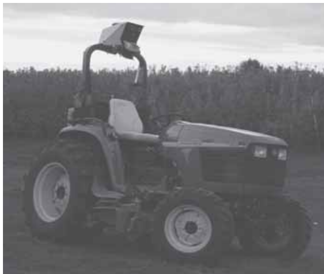
1: A John Deere tractor (4710 series) was used for some of the experiments in agricultural applications. It was equipped with cameras, positioning sensors, a computer and a SICK laser for perception.
