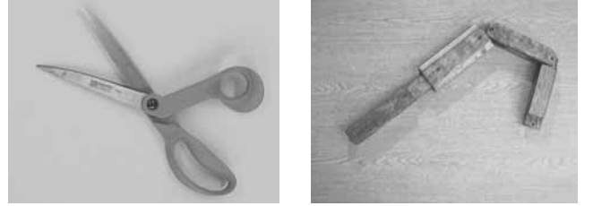
Fig. 2. Two examples of kinematic structures: scissors with a single revolute joint and a wooden toy with a prismatic joint and two revolute joints.
