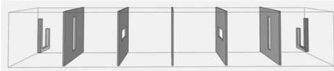
Fig. 1. A motion planning problem that can be solved more efficiently by M-sum planner. The workspace is composed of five parallel walls with horizontal and vertical windows. M-sum planner takes advantage of
