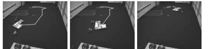
Fig. 12. Snapshots of cooperative manipulation of the L-shape part with two robots
