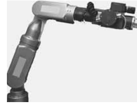
Fig. 7. The setup for the well-controlled experiments consists of the gigabit ethernet camera mounted onto a 7DOF robotic arm.
