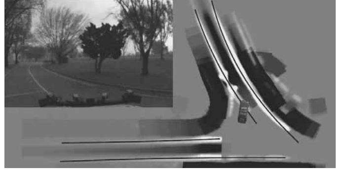
Fig. 6. The second stage of our system constructs a centerline evidence image. Lane centerline candidates (blue) are identified by fitting parabolic segments to the ridges of the image. Front-center camera is shown in top left for context.
