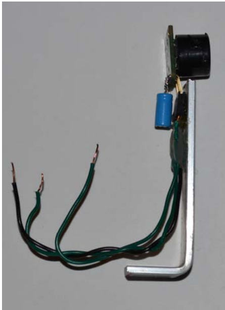
Figure 5-16. This image shows the sensor glued to the sensor bracket.
