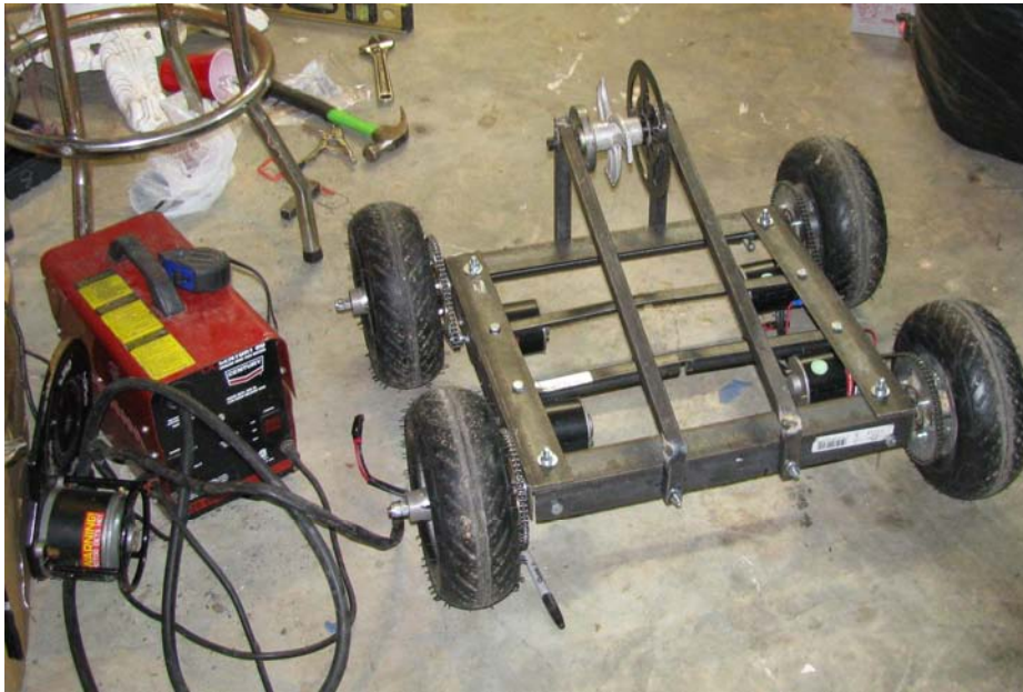
Figure 12-28. The frame with the weapon brackets and axle test-fitted
