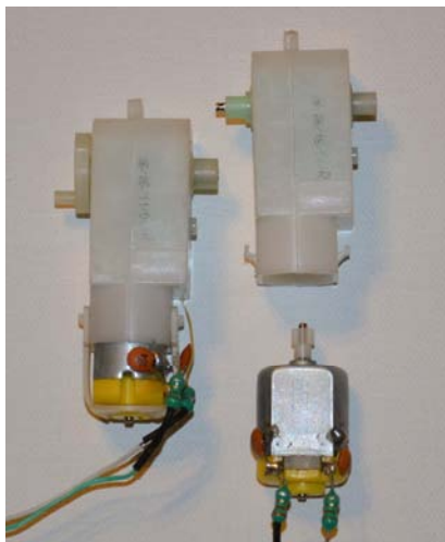
Figure 3-5. Here you can see a small DC gear motor (left) and again with the DC motor removed from the plastic gear box.
