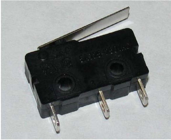
Figure 2-21. A typical tactile bump-switch with lever
