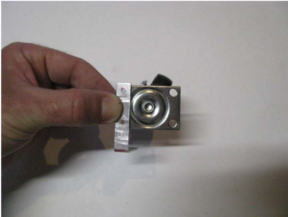
Figure 4-24. Drill holes through “L” bracket where marked.
