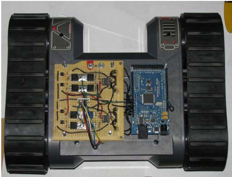
Figure 5-13. The frame base with motor-controller and Arduino mounted
