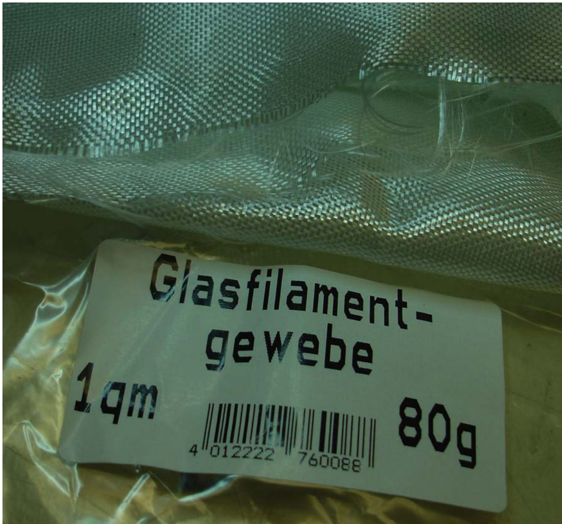
Figure 9-2. Woven fiberglass fabric with 80g/m 2
