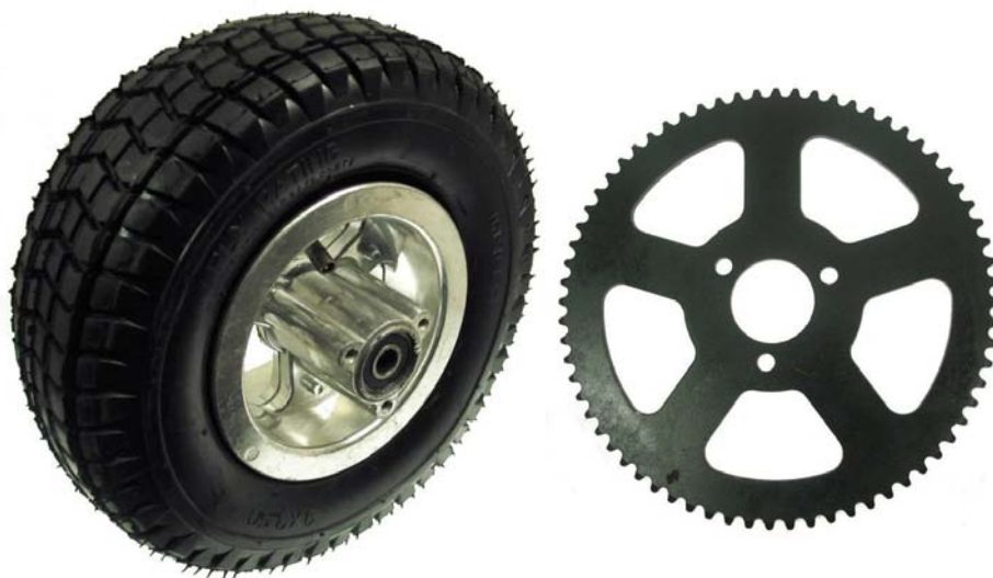
Figure 12-8. A wheel-and-sprocket pair, perfect for the Battle-bot
