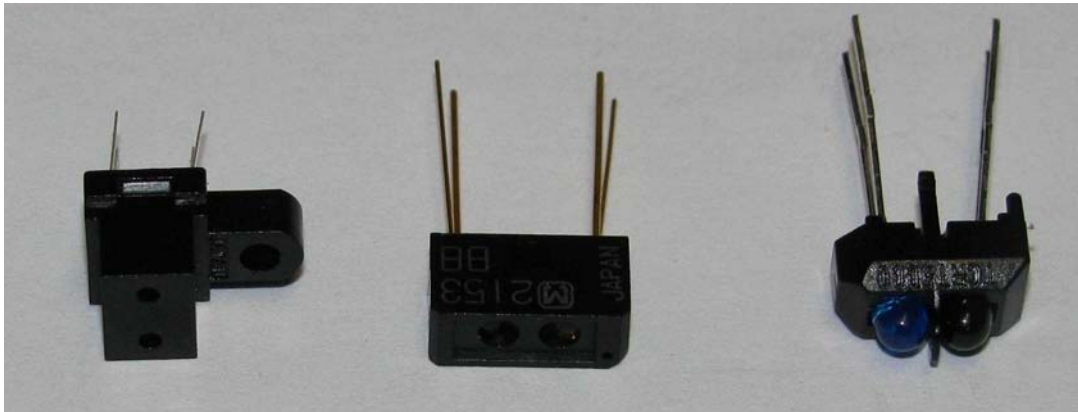
Figure 2-23. These are three different types of infrared emitter and detector pairs. The IR pair on the far right is the type used in Linus, the line-following robot from Chapter 4. These sensors range in price from $1 to $3 each from Digikey.com.
