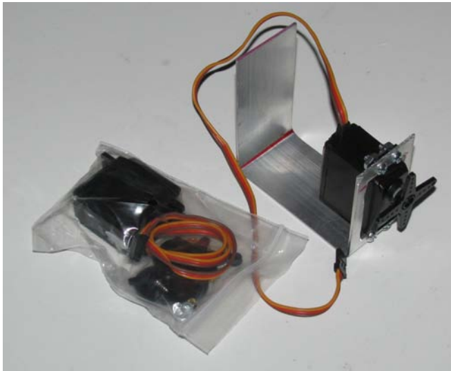
Figure 8-21. Mount the servo motor into the first aluminum bracket.
