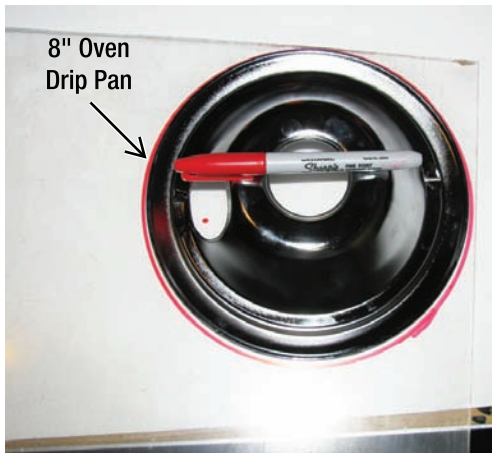
Figure 7-9. Mark a circle on the plexiglass using a permanent marker and a 6-inch to 8-inch round tin, bowl, or any object the size you would like your frame to be. If you are artistic, you might freehand a design to cut out for your frame.
