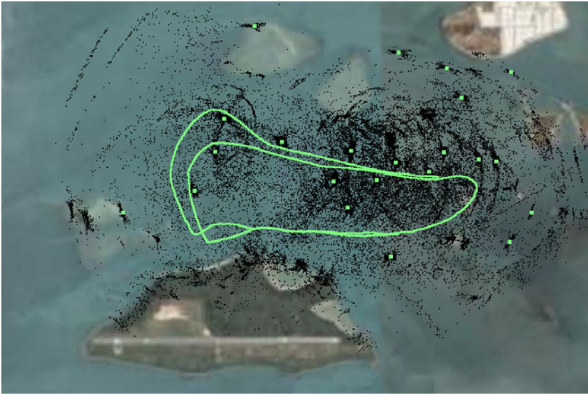
Fig. 6.15 Overview of the test site ( 1^{\circ}13' \text{ N}, 103^{\circ}43' \text{ E} ), showing the GPS trajectory (green line) and GPS coordinates-ordinates (green dots) of the point feature map. The point feature measurement history is also provided (black dots).
